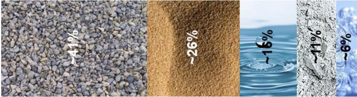
Figure 1-1. Basic ingredients of typical concrete by mass.
