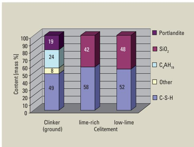
Figure 2: Calculated phase compositions of fully hydrated clinker (calculated from Taylor [8], p. 219, Aft and Afm as C<sub>4</sub>AH<sub>13</sub>) and of low-lime and lime-rich Celitement in mass %
